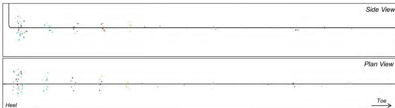
Figure 13: Synthetic microseismic events for the “no diverter” model. Only the first half length of the lateral (28 perforations) is shown.
